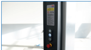
Second control unit on opposite column means less walking around the lift.
