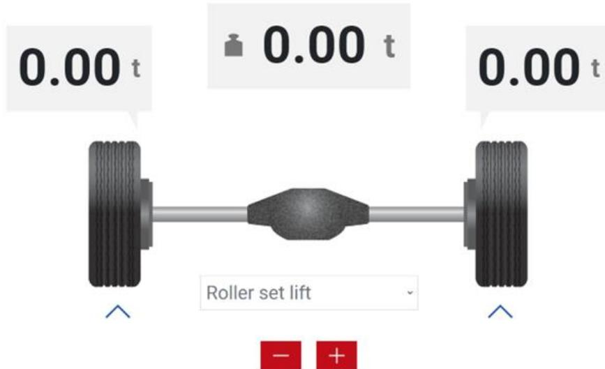
Here, the wheel weights are displayed above the wheels, and the axle weight is displayed above the axle.
