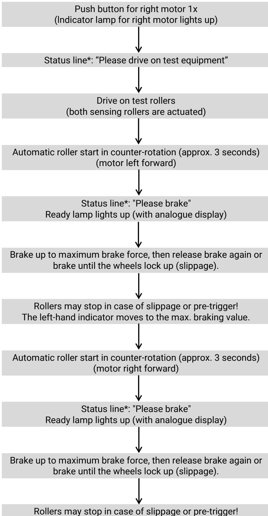
The right-hand indicator moves to the max. braking value.
